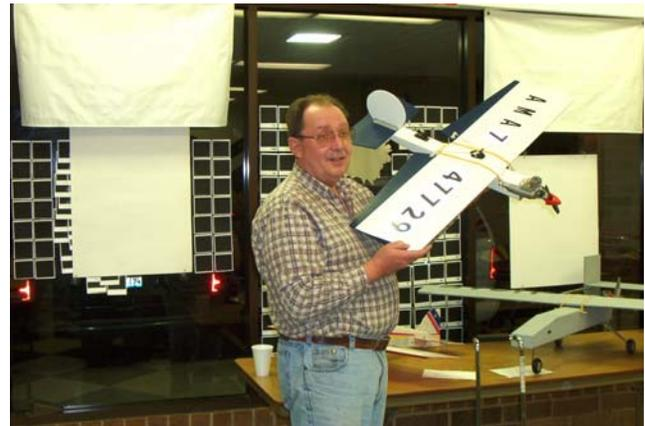
Tom Densmore brought in his Top Flight Kit built T-34 Mentor with tri gear which was work in progress and will be powered by a Saito 100 engine. ———>
